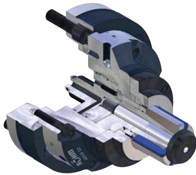
C 18 ABSIS Segment clamping mandrel, power-operated with flanged seat Consisting of basic mandrel, adapter, ejector ring, locking belt
